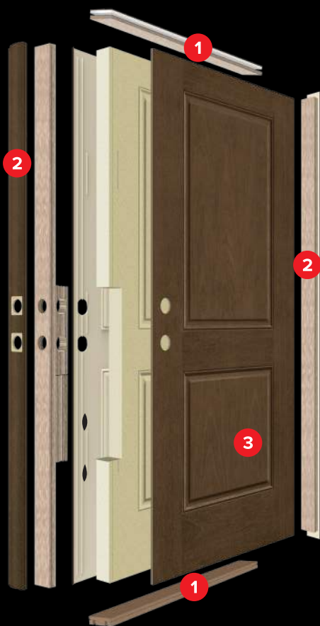
1. Top and Bottom Rails are composite for edge to edge protection. Top Rail includes LVL reinforcement for rigidity.
