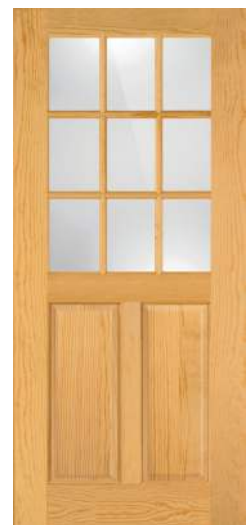
P944 Single Pane 1-5/16" TDL Bar 1-3/16" Double Hip Raised Panel Ovolo Sticking
