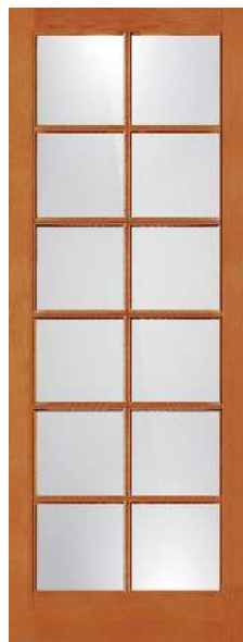
F1512 Single Pane Safety Glass 1-1/4" TDL Bar Ovolo Sticking
