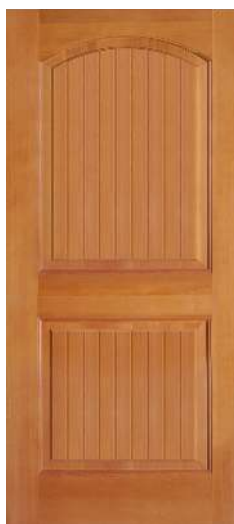
F7304 1-7/16" Beaded V-Groove Double Hip Raised Panel Wide Layout, Ovolo Sticking 3/0 x 6/8 3/0 x 8/0 3/0 x 7/0
