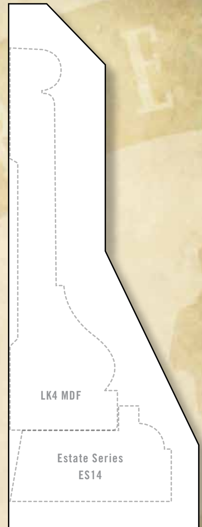
PB550 2 x 5-1/2 Will accommodate all casings and most casing/ backband combinations 4-7/8" to 5-1/4"
